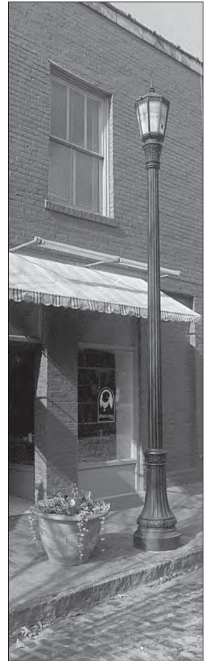
Compatible replacement streetlighting pole and fixture.
